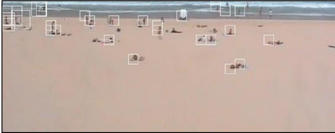
Figure 1. Image showing areas (rectangles) that have been classified as a “person object”. (Source: CoastalWatch, 2007)
