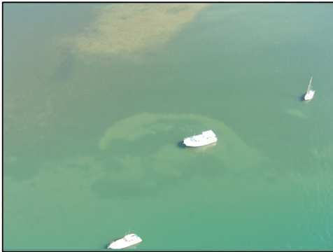
Plate 1. Aerial perspective of impacts of a traditional block and tackle mooring on seagrass habitats in Moreton Bay. Note disturbance 'halo'.
