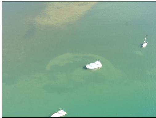
Plate 1. Disturbance halo of traditional block and tackle mooring on seagrass habitats in Moreton Bay.
