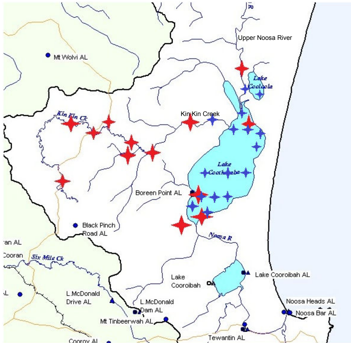
Figure 1: Suspended sediment and grab sample sediment sites from Kin Kin Creek catchment and Upper Noosa River catchment. Red stars represent water and sediment grab sample sites, while blue stars represent sediment core collection sites (Map from Bureau of Meteorology's river and flood monitoring sites for South-East Queensland, 2011).
